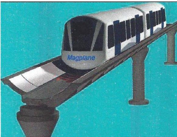
Figure 1: 30 meter trough-like concrete span with surface mounted levitation sheets and a motor winding directly below the vehicle.
