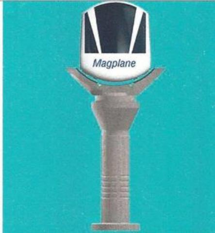
Figure 3: End-on view illustrating the large operating gap.
