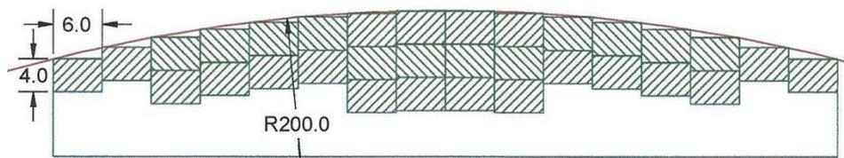
Figure 8: Optimized Cross-section Propulsion Magnet
