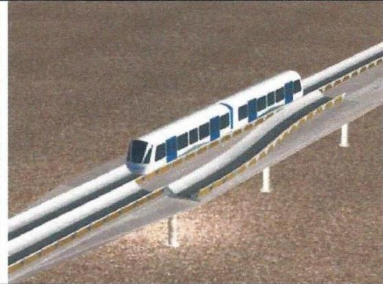
Figure 11: Mechanical Switch
