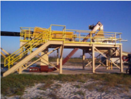
Figure 7: Load-Unload stations and transfer conveyor.
