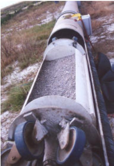
Figure 3: Car with 300 kg of phosphate rock
