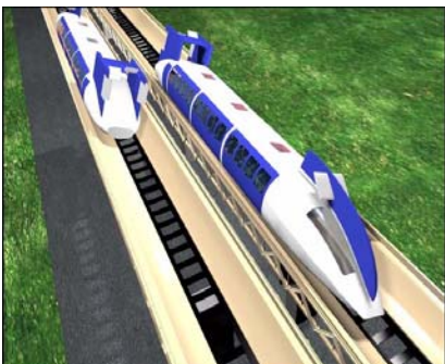
Figure 9: Passive banking in curves of +/- 10 degrees
