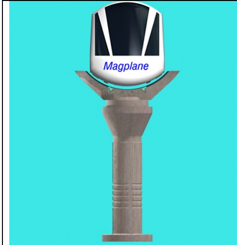
Figure 3: End-on view illustrating the large operating gap.
