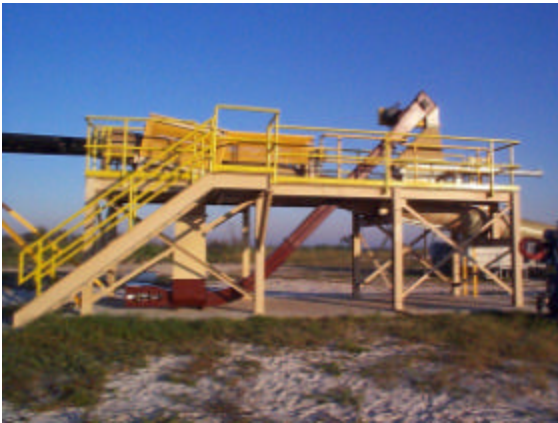
Figure 7: Load-Unload stations and transfer conveyor.
