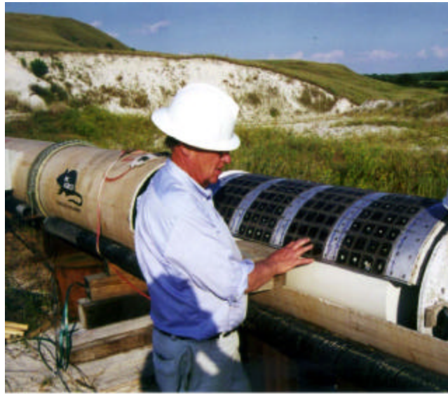
Figure 4: Magnet assembly rotated 180 degrees for inspection purposes
