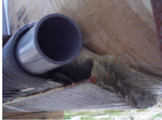
Figure 6: Close-up of LSM winding showing end turns and back iron
